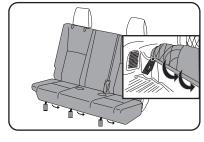
8 Locate the push clips on the front of the bottom seat cover and inset the clips inside the side seat crevice.
