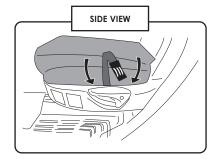
(4) Locate the push clips on the outer sides of the bottom seat covers and inset the clips inside the side seat crevice.
