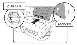
(2) Push the straps through the seat crevice to the back. Then, lift and open the original seat's flap by detaching the 2 straps from the bottom of the seat (as shown in the left corner image). Next, pull the seat cover straps and attach them to the seat's upholstery, reattach the seat's flap and attach the cover's back hook-and-loop attachments to the seat. Repeat the same process to install the other backrest.
