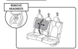
(1) To start, remove all headrests by pushing on the release button at the base of the headrests. Next, take the 2-Row Backrest (60 side) seat cover, unzip it and slide it over the bigger backrest making sure the cover goes under the middle seat seatbelt. Then, accommodate the cover so it follows the shape of the backrest and zip it together on the back of the seat.
