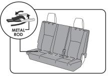
7 To install the bottom seat cover, place the cover on the seat following the seat's shape. Then, attach the cover straps to the metal rod inside the seat crevice (just as you attached the backrest straps).
