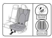
(3) To Install the 60 and 40 side bottom seat covers, place each cover on the bottom seat respectively. Then, push the buckle straps through the seat's crevice and connect them to the front straps underneath the seat as shown in the image.
