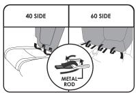
(a) Locate the metal rod inside the seat crevice and attach the seat cover straps around the rod as shown in the picture. Make sure to secure the straps with the hook-and-loop adhesives.
