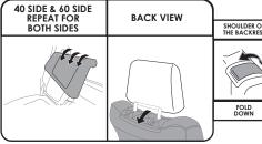
(5) Slide the 3-Row backrest covers over each backrest. TIP: Folding down the backrest will make this process easier. Once the covers are on, close the headrest opening and secure the back of the cover using the hook-and-loop attachments.
