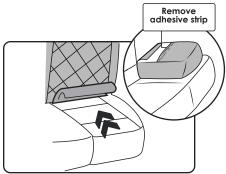
(3) Locate the fabric flap at the bottom of the 40 side backrest cover and push it through the seat's crevice. Then, attach it to back side of the seat cover.
