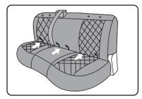
6 Place the bottom seat cover on the bench seat cushion and push the buckle straps through the center crevice of your car seat.
