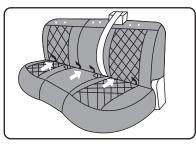
6 Place the bottom seat cover on the bench seat cushion and push the buckle straps through the center crevice of your car seat.
