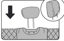
(8) Slip on the headrest cover and reattach the headrests. TIP: Starting from either side of the headrest and sliding the cover sideways will help you achieve a secure fit.
