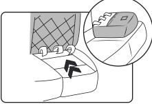
(3) Push the hook-and-loop straps located on the bottom of the left backrest cover through the seat crevice. Attach the rear hook-and-loop straps directly to the upholstery on the back of the seats.
