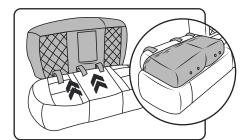
(5) Push the hook-and-loop straps located at the bottom of the right backrest cover through the seat crevice. Attach the rear hook-and-loop straps directly to the upholstery of the back seats.
