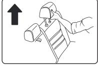
To start, remove the headrest by pushing the release button at the base of the headrest.
