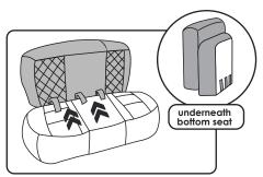
(4) Push the rear hook-and-loop straps through the seat crevice. Lift up the bottom seat and attach the rear hook-and-loop straps underneath the bottom seat.
