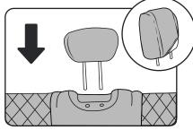
(8) Slip on the headrest cover and reattach the headrests. TIP: Starting from either side of the headrest and sliding the cover sideways will help you achieve a secure fit.
