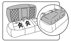
Push the rear hook-and-loop straps through the seat crevice. Attach the rear hook-and-loop straps directly to the upholstery of the backseats.
