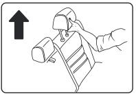
1 To start, remove the headrest by pushing the release button at the base of the headrest.
