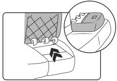
(3) Push the hook-and-loop straps located on the bottom of the left backrest through the seat crevice. Attach the rear hook-and-loop straps directly to the upholstery of the backseats.
