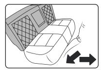
6 Remove the bottom seats by pushing diagonally inward then pulling the bottom bench seat cushion up and out.
