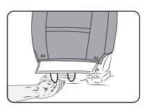
3 On the lower part of the back of the seat, detach the seat's flap by removing the clips underneath the seat. That way, you will expose the underside of your seat.
