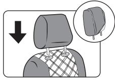
(8) Slip on the headrest cover. TIP: Starting from either side of the headrest and sliding the cover sideways will help you achieve a secure fit. Finally reattach the headrest to the top of the car seat.
