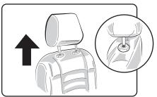
1 Detach the headrest by pressing the button located at the base of the headrest. Then simply lift the headrest to separate it from the backrest.
