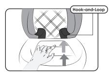
4 Push the straps through the seat crevice, and position the straps to the back of the seat.
