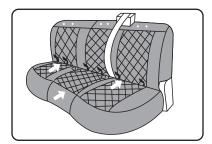
(5) Place the Bottom 60 and 40 Side covers on the bench seat cushion and push the buckle straps to the center crevice of your car seat.
