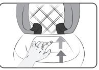
(3) Push the straps through the seat crevice, and position the straps to the back of the seat.
