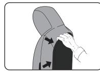
② Once the backrest is pulled down, carefully tuck in the excess car seat cover fabric into the crevice of the rear panel on the Tesla car seat. Use a plastic tool to assist with tucking the seat cover in neatly.
