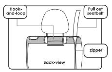
(2) After you successfully place the seat cover over the backrest, slide the piece of fabric underneath the headrest and attach the hook-and-loop to the back of the seat. Also, make sure you unzip the zipper and pull out the seatbelt as shown in the image above.
