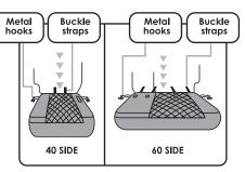
6 For the split bench Tesla, place the bottom 60 and 40 side covers on each seat bottom and push the buckle straps to the center crevice of your car seat.
