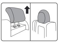
Slip on the headrest cover and reattach the headrests. TIP: Starting from either side of the headrest and sliding the cover sideways will help you achieve a secure fit. Repeat same process for all headrests.
