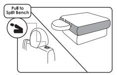
Slide the backrest driver side cover onto backrest following the contour of the seat, until it's fully on the backrest. Then, close the hook-and-loop straps near the seatbelt holder and tuck in the reminder fabric in the seat crevice. Repeat this process with the passenger side backrest.
