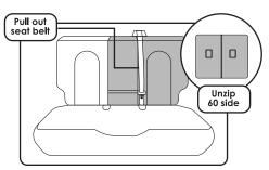
4 Pull the 60 side backrest forward, unzip the backrest cover and slide it onto the backrest. Make sure you pull out your vehicles seat belt before you zip up the backrest cover.
