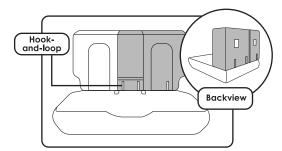
(5) Push the hook-and-loop straps through the seat crevice. Then, attach them directly to the upholstery of the backseats.
