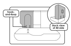
3 Push the hook-and-loop straps through the seat crevice. Then, attach them directly to the upholstery of the backseats.
