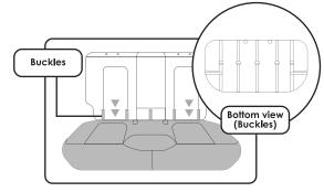
Place the bottom seat cover on the bench seat cushion and attach the buckles as shown above. Once completed, reattach the bottom of the seat to the vehicle.
