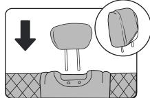
(8) Reattach the headrests on and slip on the headrest covers. TIP: Starting from either side of the headrest and sliding the cover sideways will help you achieve a secure fit.
