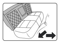
(6) Remove the bottom of the seat by pushing diagonally inward then pulling the bottom bench seat cushion up and out
